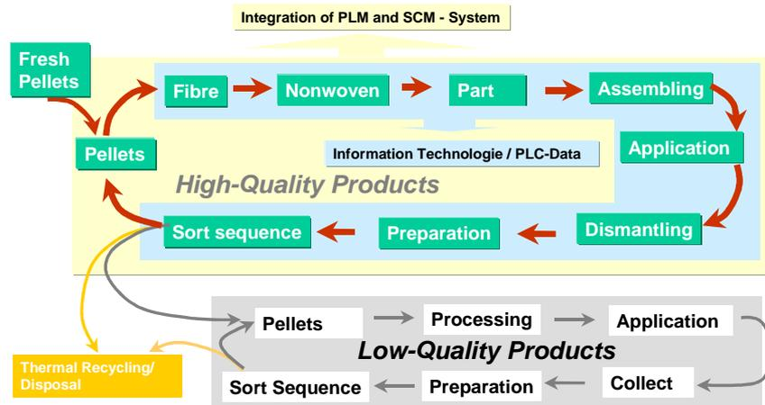
Figure 6. The Controlled Closed Loop Recycling
