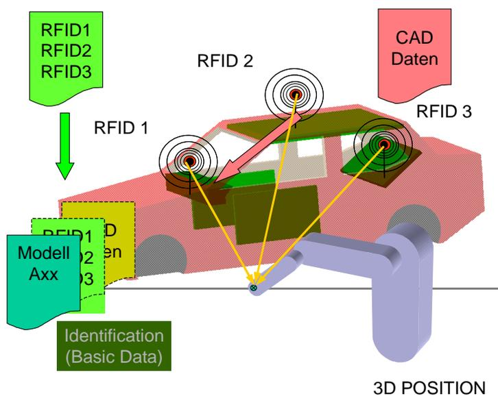
Figure 8. Scheme of Triangulation-principle for easy dismantling
