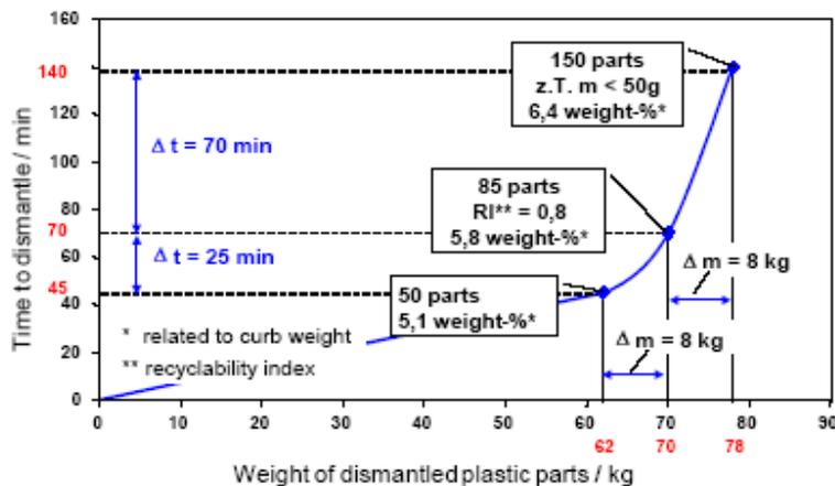
Figure 7. Dismantling of plastic components in end-of-life vehicles [3]
