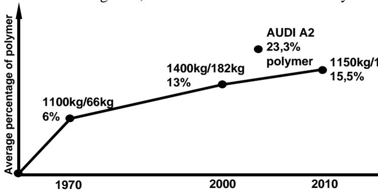
Figure 1. Average percentage of polymer automotive parts [1]
