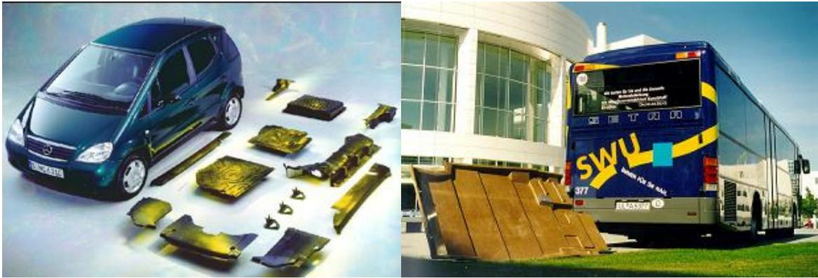
Figure 3. Current examples of fibre reinforced material applications
