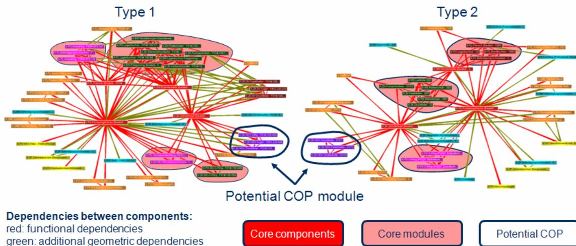
Figure 4. Structural comparison of types of high pressure pump for identification of COP potential
