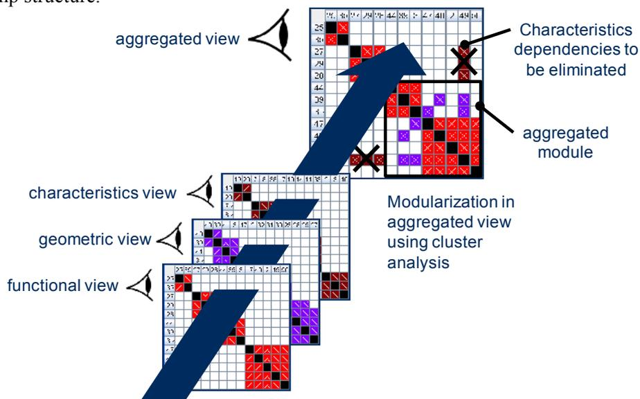
Figure 3. 3D-Clustering of component dependencies, derived from Multiple-Domain Matrix
