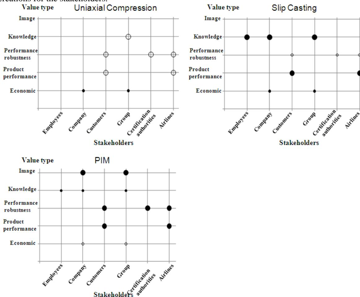
Figure 3. Stakeholders/expected values for uniaxial compression, slip casting and PIM process. Value creations range from Very low value creation (big empty dot) to very high value creation (big full dot)
